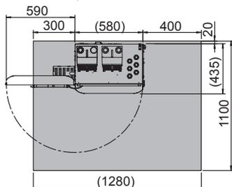
\*4: Required clearance needed for wiring.
