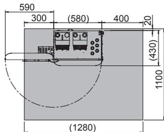
\*5: Required clearance needed for wiring.
