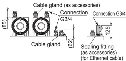
For FM-X, CSA-X (wiring connection: 3/4NPT)
