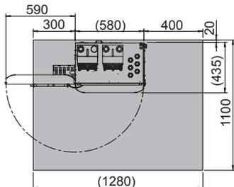
\*4: Required clearance needed for wiring.
