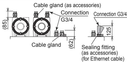
For FM-X, CSA-X (wiring connection: 3/4NPT)
