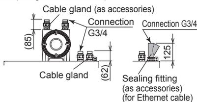
For FM-X, CSA-X (wiring connection: 3/4NPT)
