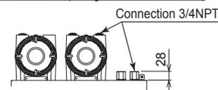
For FM-Y, CSA-Y (wiring connection: 3/4NPT)
